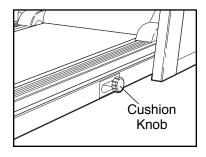
knob on the right side of the treadmill. For a firmer walking platform, turn the knob counterclockwise. For a softer walking platform, turn the knob clockwise. Note: The faster you run on the treadmill, the firmer the walking platform should be. If the walking platform is too soft, the treadmill may bounce excessively.
